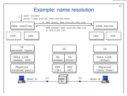
Flow 2 illustrates the query/response protocol of the Domain Name System (DNS). The name resolver and the name server are two application programs, probably C programs making calls to the socket library. The programs use UDP, which is the non-reliable transport protocol in the TCP/IP stack.
