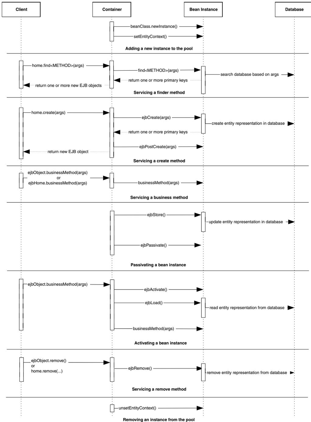
**Figure E.10** Sequence diagram for bean managed persistent entity beans. For simplicity, the Container object represents all container subsystems, including EJB objects, home objects, transaction services, and so on.
