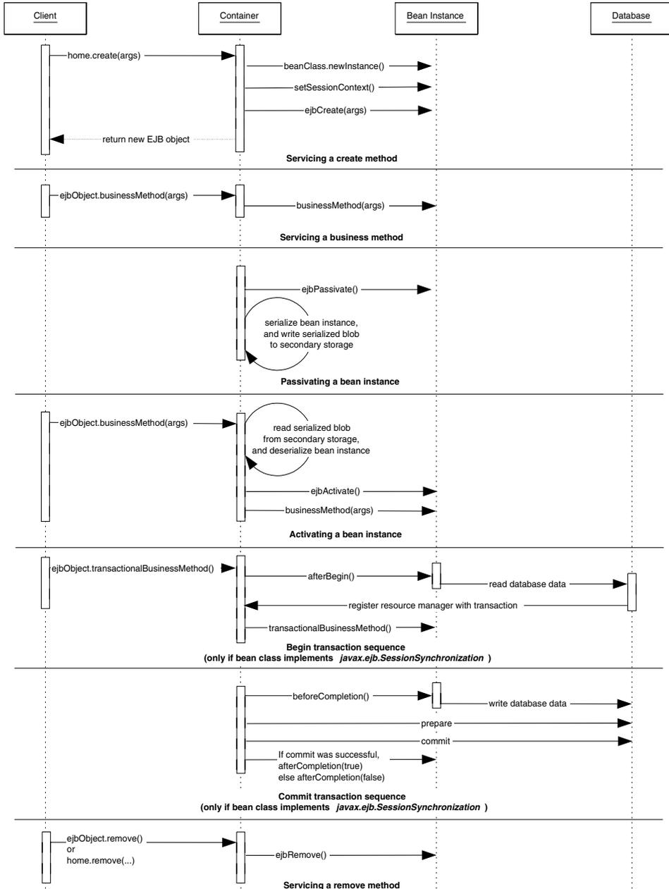
**Figure E.6** Sequence diagram for stateful session beans. For simplicity, the Container object represents all container subsystems, including EJB objects, home objects, transaction services, and so on.
