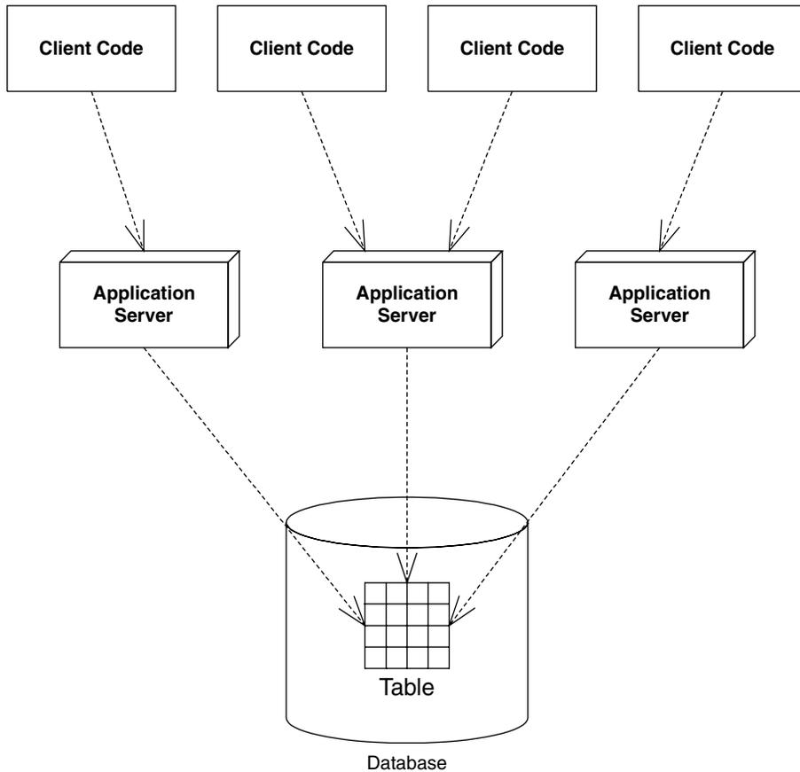
**Figure 10.2** Application servers tied to a single database.
