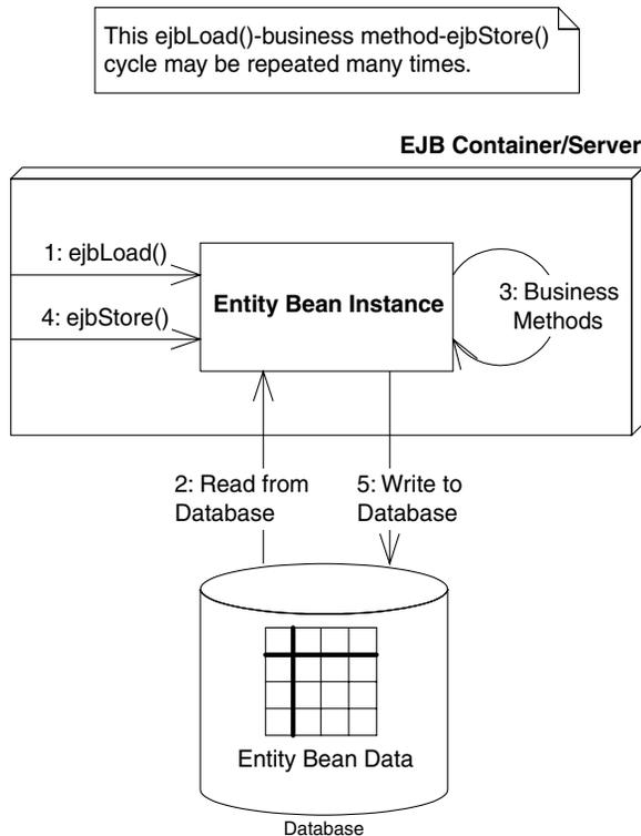
**Figure 5.3** Loading and storing an entity bean.
