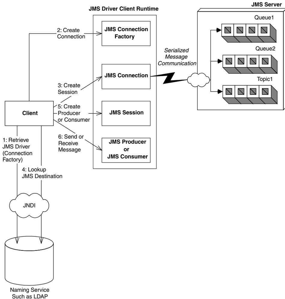
**Figure 8.3** Client view of a JMS system.
