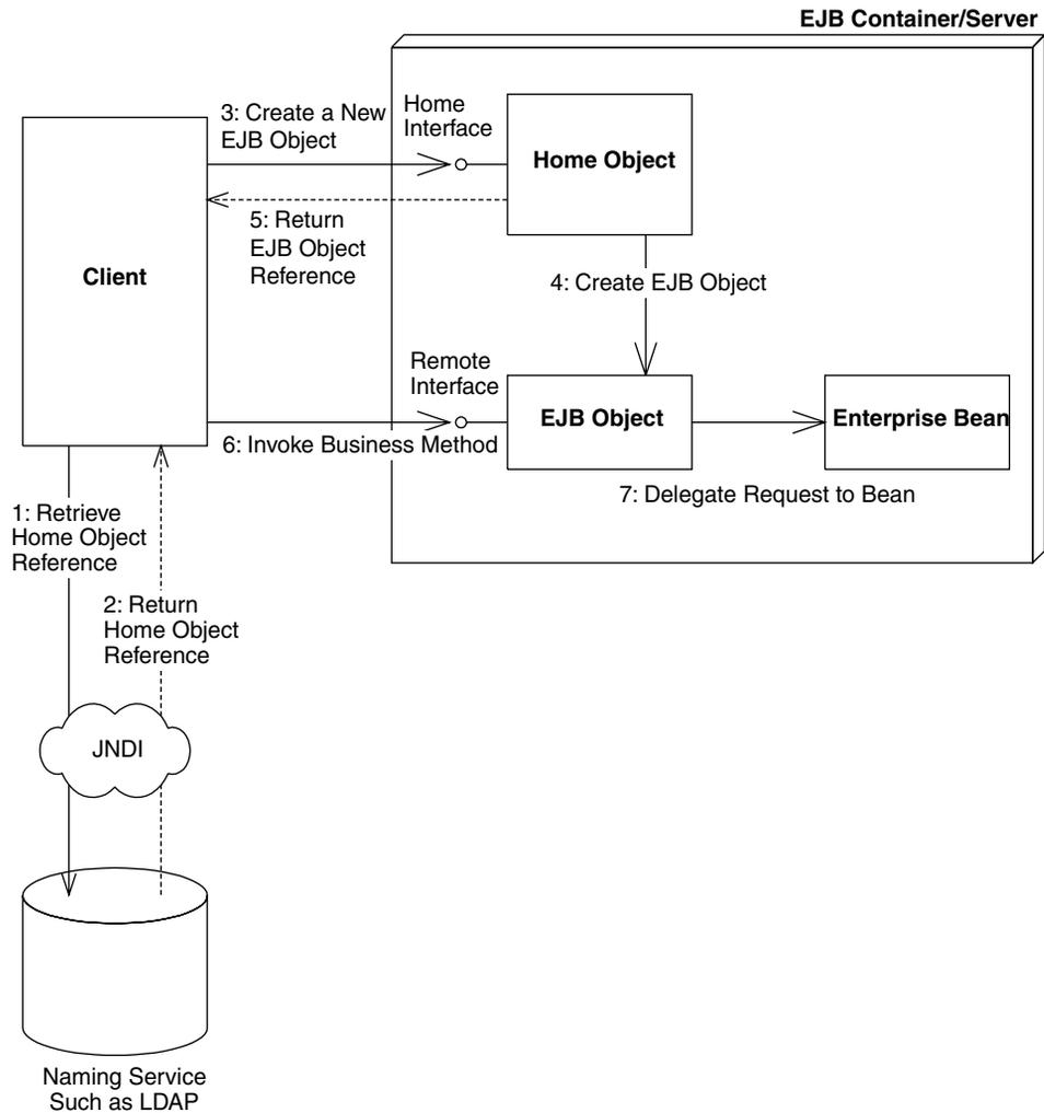
**Figure 3.3** Acquiring a reference to a home object.
