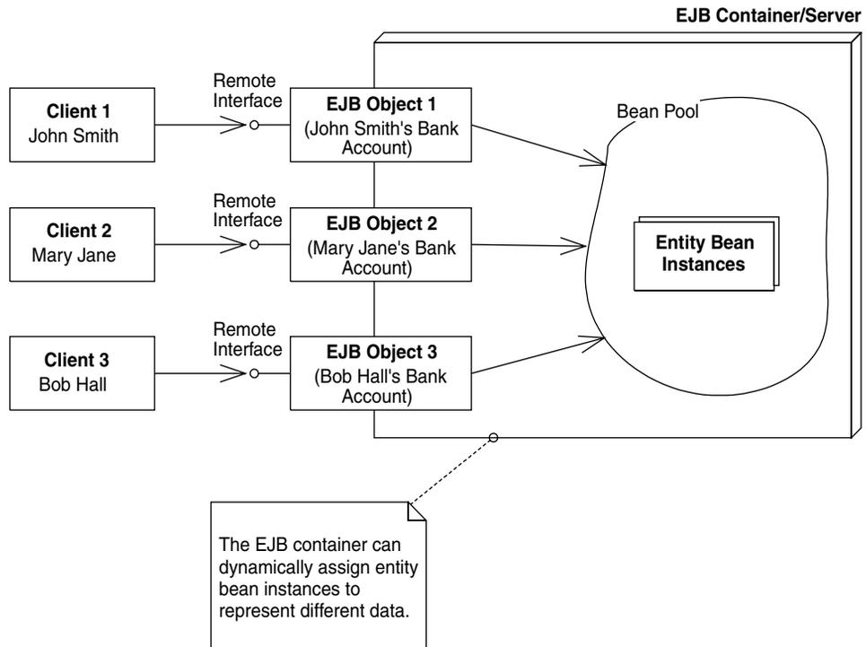
**Figure 5.4** EJB container pooling of entity beans.
