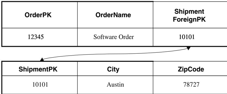
**Figure 11.2** A possible one-to-one cardinality database schema.
