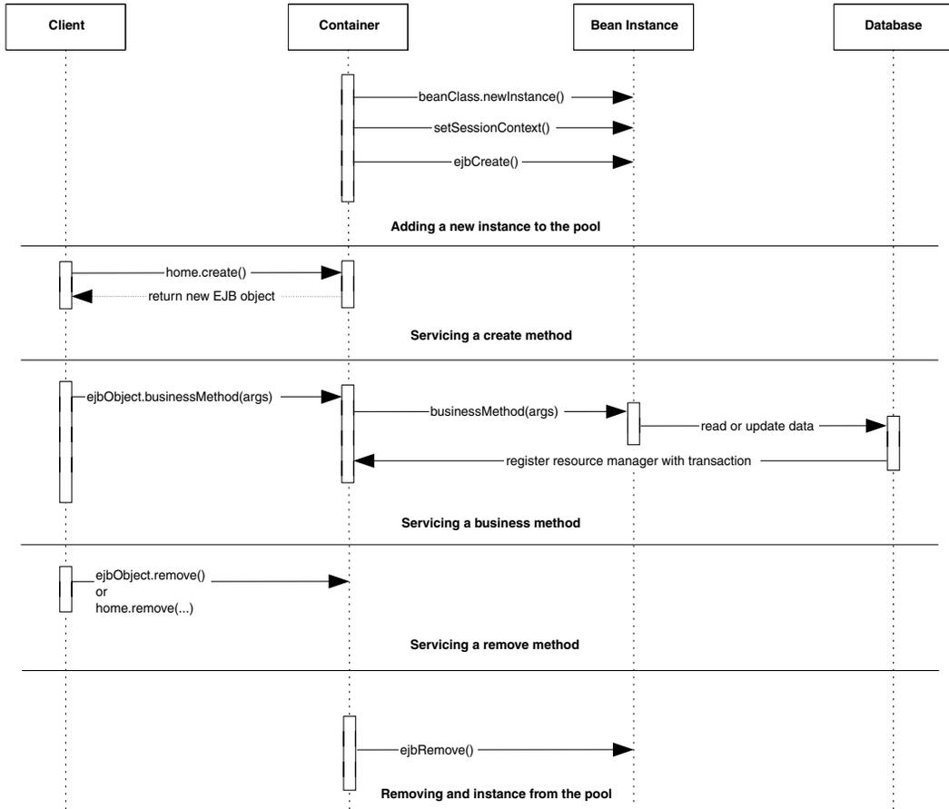
**Figure E.3** Sequence diagram for stateless session beans. For simplicity, the Container object represents all container subsystems, including EJB objects, home objects, transaction services, and so on.
