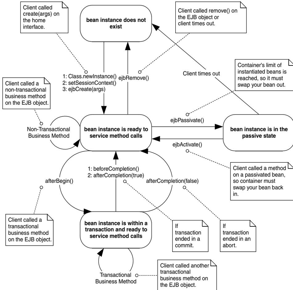
**Figure E.5** The life cycle of a stateful session bean (implements *javax.ejb.SessionSynchronization*). Each method call shown is an invocation from the container to the bean instance.
