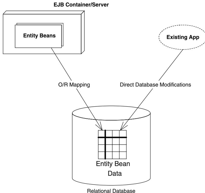
**Figure 5.8** Modifying an entity bean's database representation manually.
