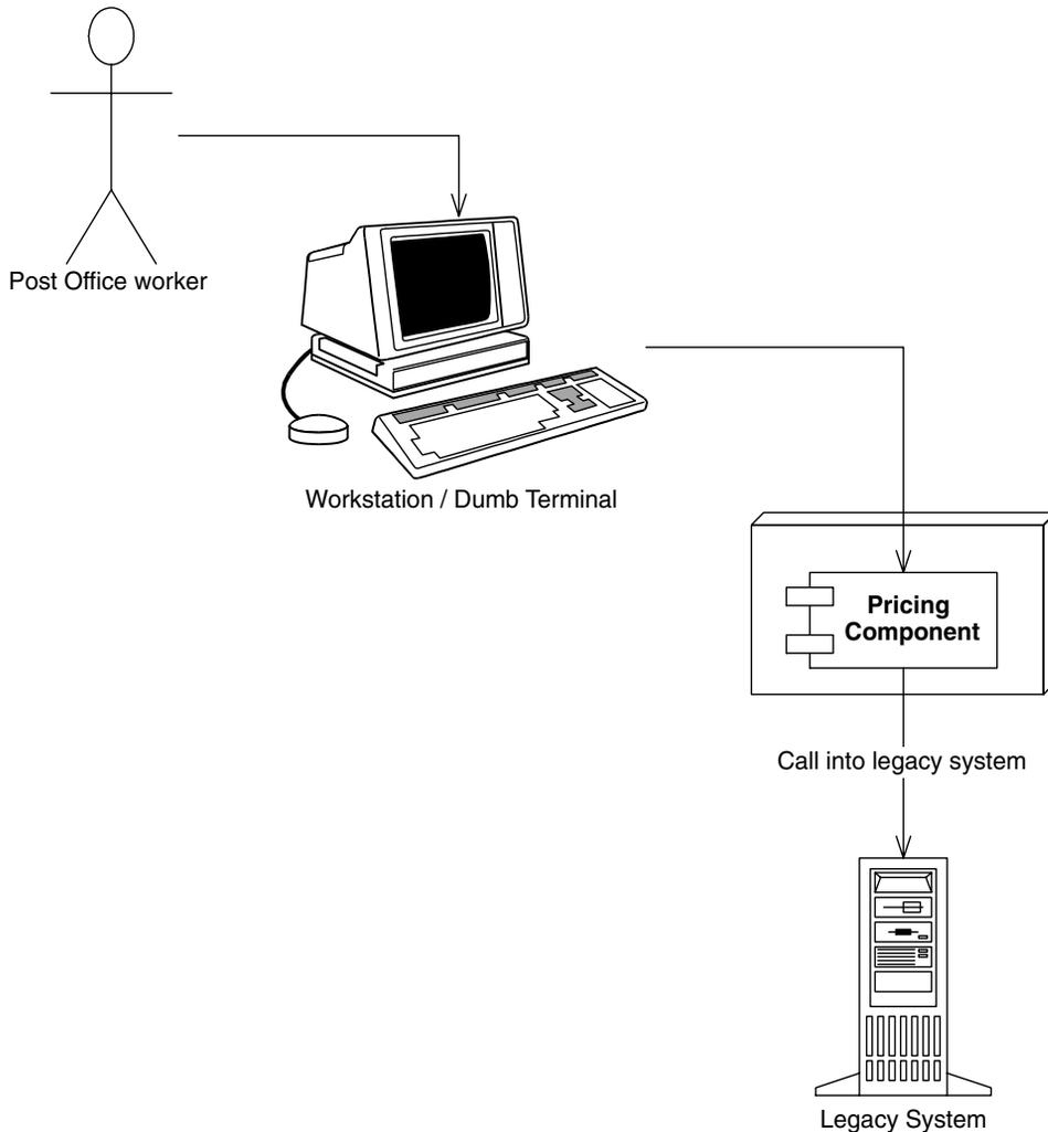
**Figure 1.2** Reusing a pricing component for the U.S. Postal Service.
