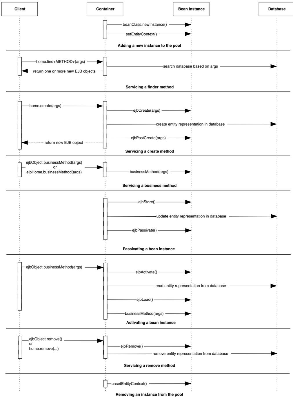
**Figure E.11** Sequence diagram for container managed persistent entity beans. For simplicity, the Container object represents all container subsystems, including EJB objects, home objects, transaction services, and so on.
