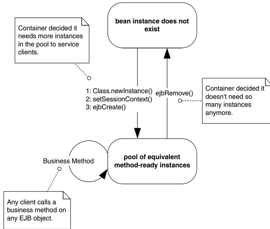
**Figure E.2** The life cycle of a stateless session bean. Each method call shown is an invocation from the container to the bean instance.
