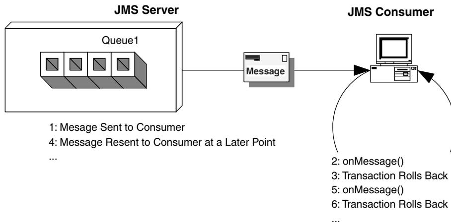
**Figure 8.7** How message-driven beans can cause poison messages.
