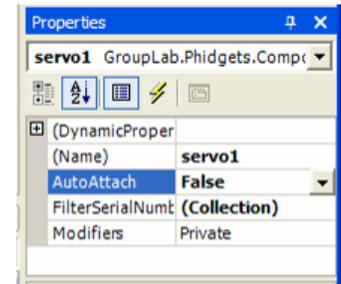
**Run the example.** The component does not attach to the Phidget Servo even though it is plugged in. The `Attach` event is not raised. Then set the `AutoAttach` property back to `True`
