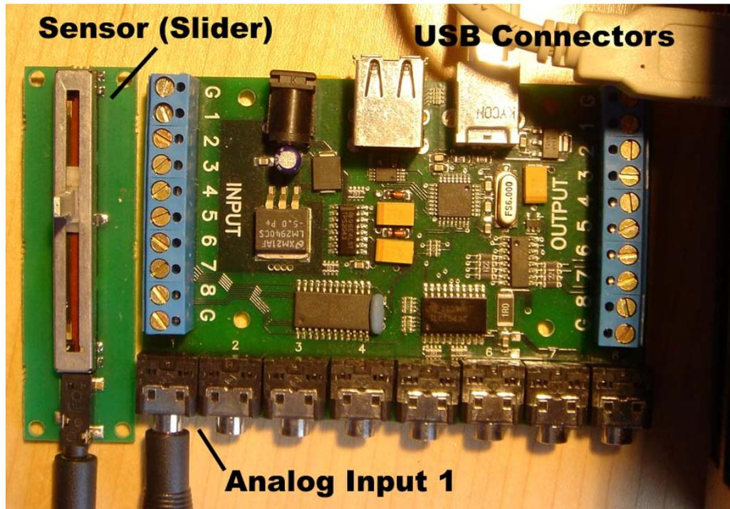
An 8/8/8 Phidget InterfaceKit, with a slider sensor plugged into Analog Input #1.
