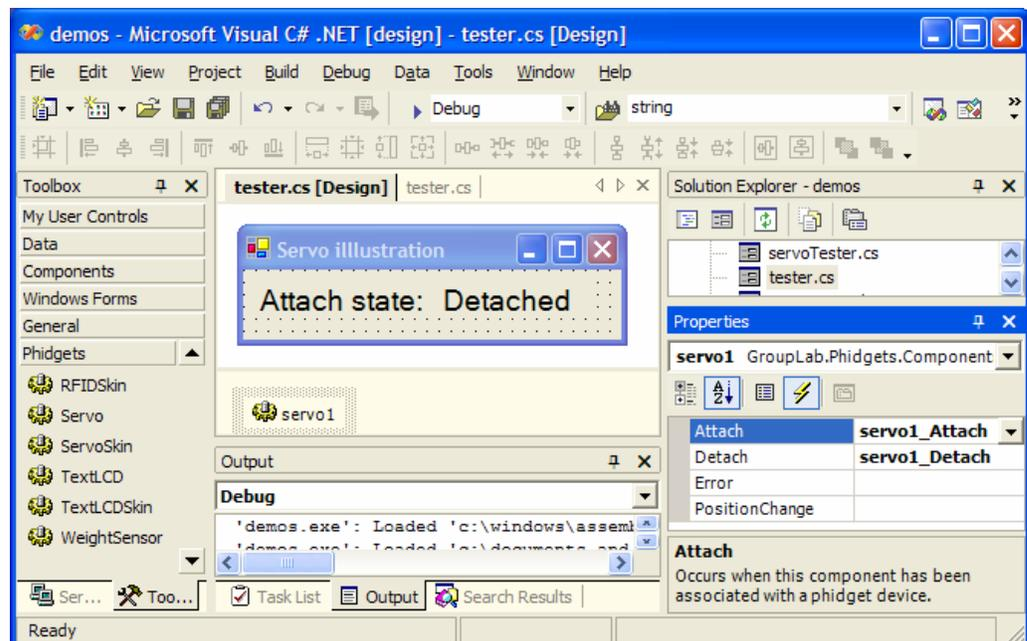
**Program the Attach event handler** via the `servo1_Attach` event handler. This is executed when the servo device is seen by the system (i.e., when you start the program if the servo is plugged in, or if you plug in the servo after the program has been started.
