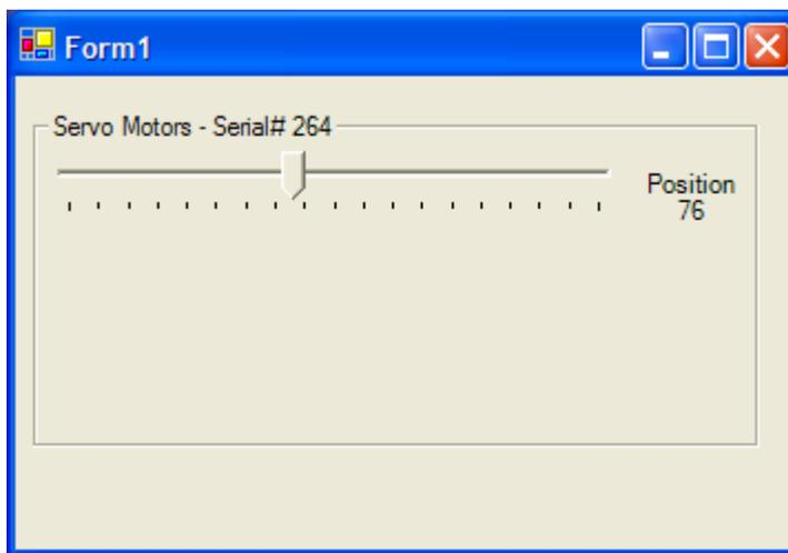
**Move the slider on the trackBar.** As you move it, the servo motor plugged into the Phidget Servo should rotate to the given angle. This angle can be between 0 to 180 degrees. The actual angle will appear on the right of the trackbar.
