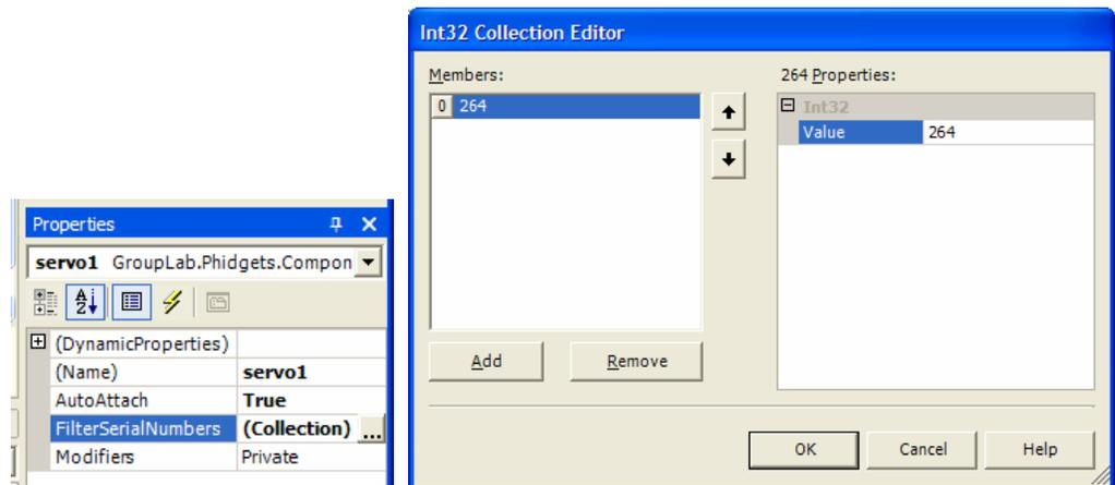
**Run the example.** The component attaches to the Phidget Servo, as you would expect. If you have a second Phidget Servo, try unplugging the first one and plugging in the second one. You will see that the other servo does not attach, as its serial number is not on the list. You can also plug both servos in, and restart the program. Again, you will see that only the phidget servo with the right serial number is included.
