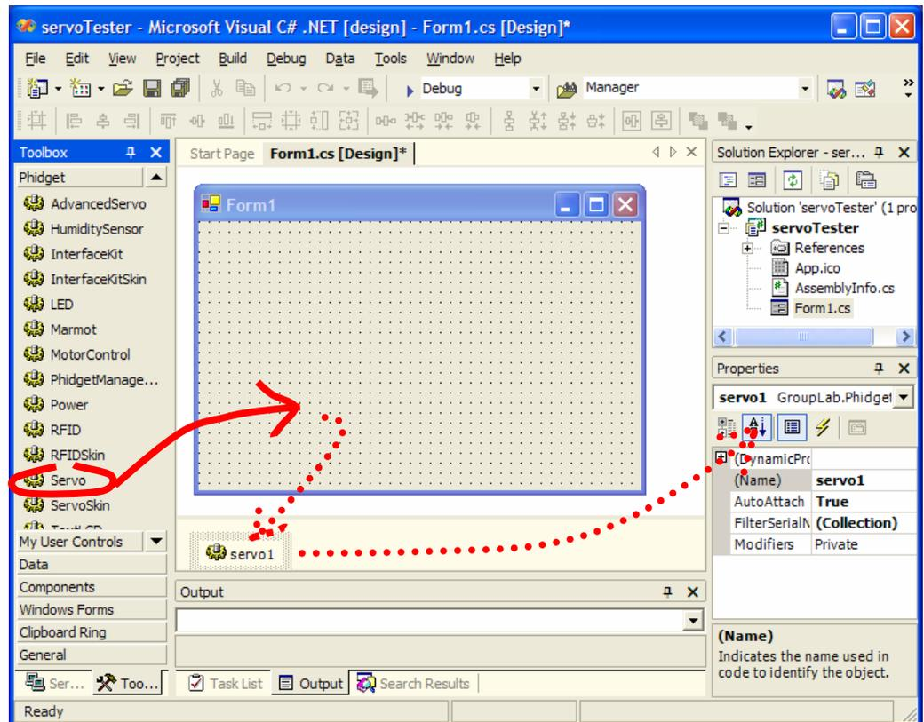
Drag and drop a Servo component into the form, and view its properties.
