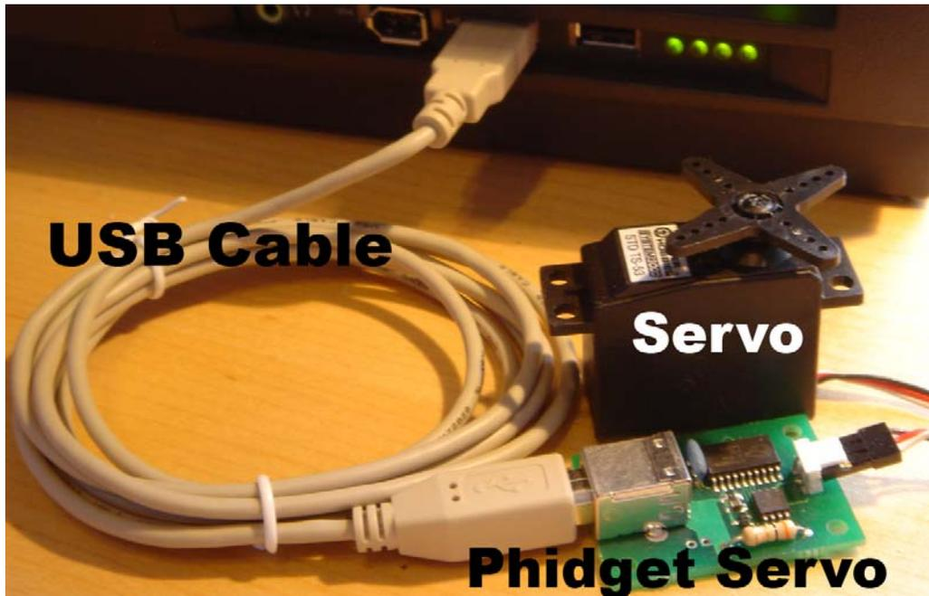
A 1-servo phidget plugged into a computer; the servo motor is also connected to the hardware board.
