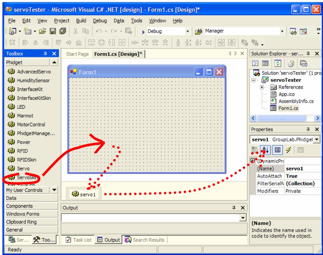
**Drag and position a ServoSkin** from the Toolbox onto the Form1 window, as illustrated in the next figure. This creates the graphical skin – a widget – that will let you see and control the servo motor. It will likely be called servoSkin1. It too is an object, but with graphical properties. Click on it to see its properties in the Properties window.
