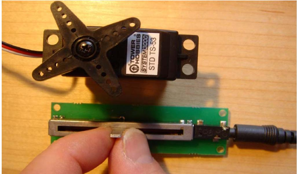
As before, plug a sensor such as a slider into Analog Input #1 of the Phidget InterfaceKit. Using the USB cable, plug the Phidget InterfaceKit into a USB port on your computer. Using another USB cable, plug the Phidget Servo into another USB port on your computer.
