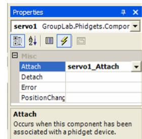
**Insert the following code in the servo1\_Attach event handler.** The Attach event is raised when the servo device is seen by the system (i.e., when you start the program if the servo is plugged in, or if you plug in the servo after the program has been started. Through the code below, the `servo1_Attach` event handler will just rotate the 1<sup>st</sup> servo motor (counting from 0) to a random position between 0 and 180 degrees by setting that motor's `Position` property.
