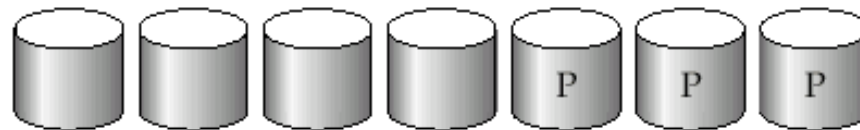
(c) RAID 2: memory-style error-correcting codes
