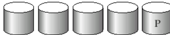
(e) RAID 4: block-interleaved parity
