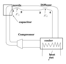
Fig. -7.4. Schematic of a supersonic tunnel in a continuous region (and also for example (7.3)
