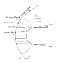
Fig. -14.14. The schematic for a round—tip bullet in a supersonic flow.
