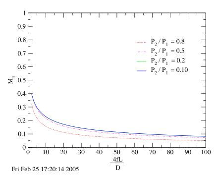
Fig. -9.3. The Mach number at the entrance to a tube under isothermal flow model as a function  $\frac{4fL}{D}$
