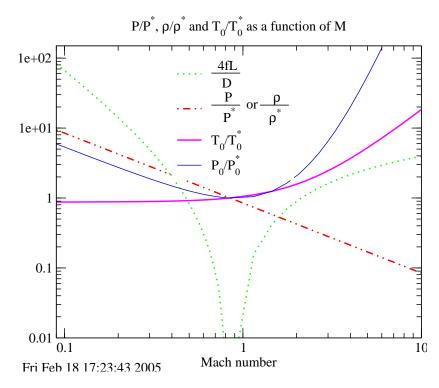
Fig. -9.2. Description of the pressure, temperature relationships as a function of the Mach number for isothermal flow
