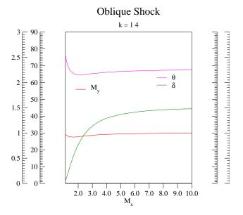
Fig. -14.18. Maximum values of the properties in an oblique shock
