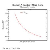
Fig. -6.16. The maximum of "downstream" Mach number as a function of the specific heat, k.
