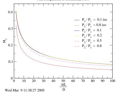
Fig. -10.21. The entrance Mach number as a function of dimensionless resistance and comparison with Isothermal Flow
