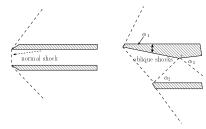
Fig. -14.19. Two variations of inlet suction for supersonic flow.
