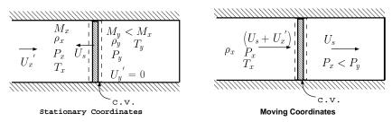
Fig. -6.9. Comparison between a stationary shock and a moving shock in a stationary medium in ducts.
