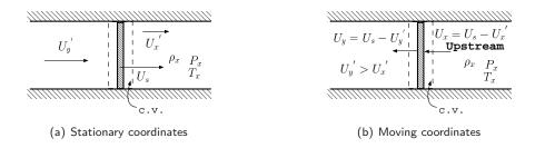
Fig. -6.18. A shock moves into a moving medium as a result of a sudden and complete open valve.
