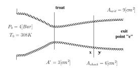
Fig. -7.2. A nozzle with normal shock
