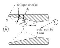
Fig. -14.16. The "detached" shock in a complicated configuration sometimes referred to as Mach reflection.
