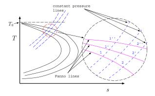
Fig. -10.7. The development properties in of converging nozzle
