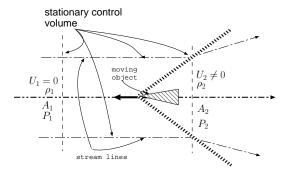
Fig. -14.23. The diagram that explains the shock drag effect of a moving shock considering the oblique shock effects.
