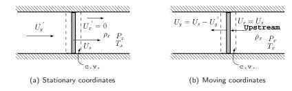
Fig. -6.12. A shock moves into a still medium as a result of a sudden and complete opening of a valve
