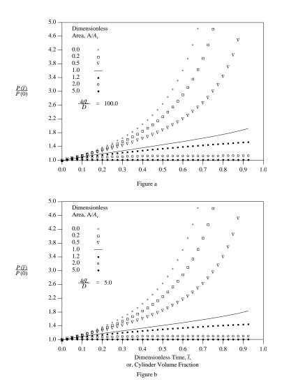
Fig. -13.2. The pressure ratio as a function of the dimensionless time for chokeless condition
