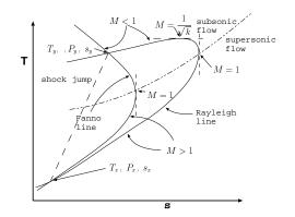
Fig. -6.2. The intersection of Fanno flow and Rayleigh flow produces two solutions for the shock wave.
