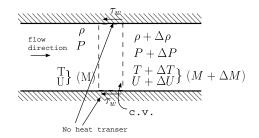
Fig. -10.1. Control volume of the gas flow in a constant cross section
