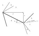
Fig. -15.8. The definition of attack angle for the Prandtl–Meyer function.
