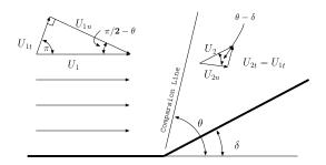
Fig. -14.3. A typical oblique shock schematic
