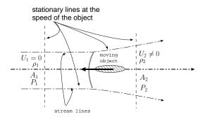
Fig. -6.7. The diagram that reexplains the shock drag effect of a moving shock.
