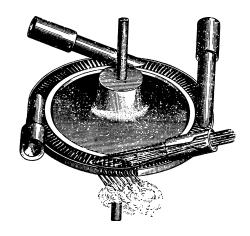
Fig. -1.2. The schematic of deLavel's turbine after Stodola, Steam and Gas Turbine
