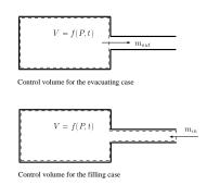
Fig. -12.3. A schematic of the control volumes used in this model
