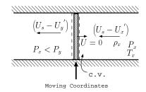
Fig. -6.6. Comparison between stationary shock and moving shock in ducts.
