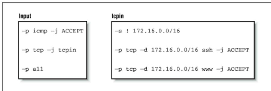
Our `input` and `tcpin` chains are populated with our rules. Datagram processing always begins at one of the inbuilt chains. We'll see how our user-defined chain is called into play by following the processing path of different types of datagrams.
