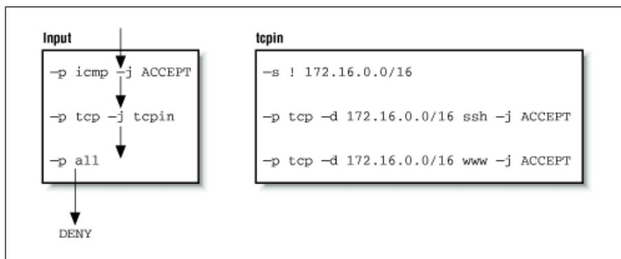
The datagram is received by the `input` chain and falls through the first two rules because they match ICMP and TCP protocols, respectively. It matches the third rule in the `input` chain, but it doesn't specify a target, so its datagram and byte counters are updated, but no other action takes place. The datagram reaches the end of the `input` chain, meets with the default `input` chain policy, and is denied.
