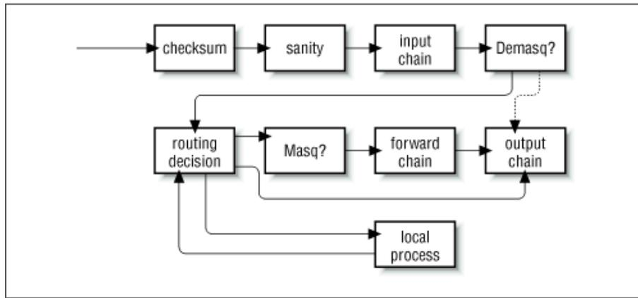
In [Figure 9.8](#), the components labeled "demasq" and "masq" are separate kernel components responsible for the incoming and outgoing processing of masqueraded datagrams. These have been reimplemented as *netfilter* modules.
