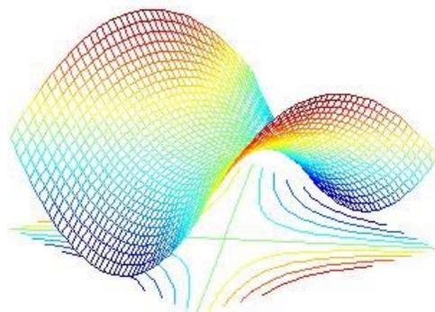
Function **surf** is used to visualize data as a shaded surface.
