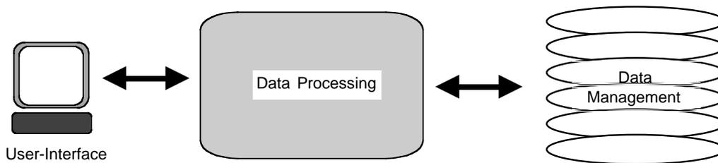
**Figure 1-1.** Functional Decomposition of an Information System
