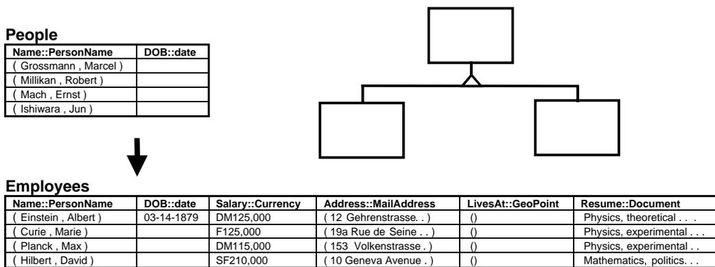
**Figure 1–3.** Inheritance in an Object-Relational Database
