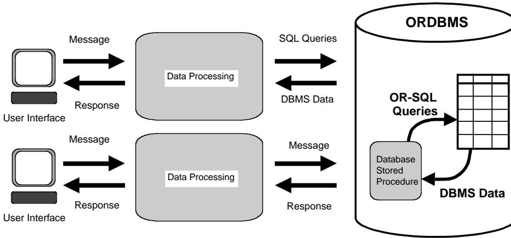
**Figure 1-5.** Routine Extensibility and the ORDBMS as the Object-Server Architecture
