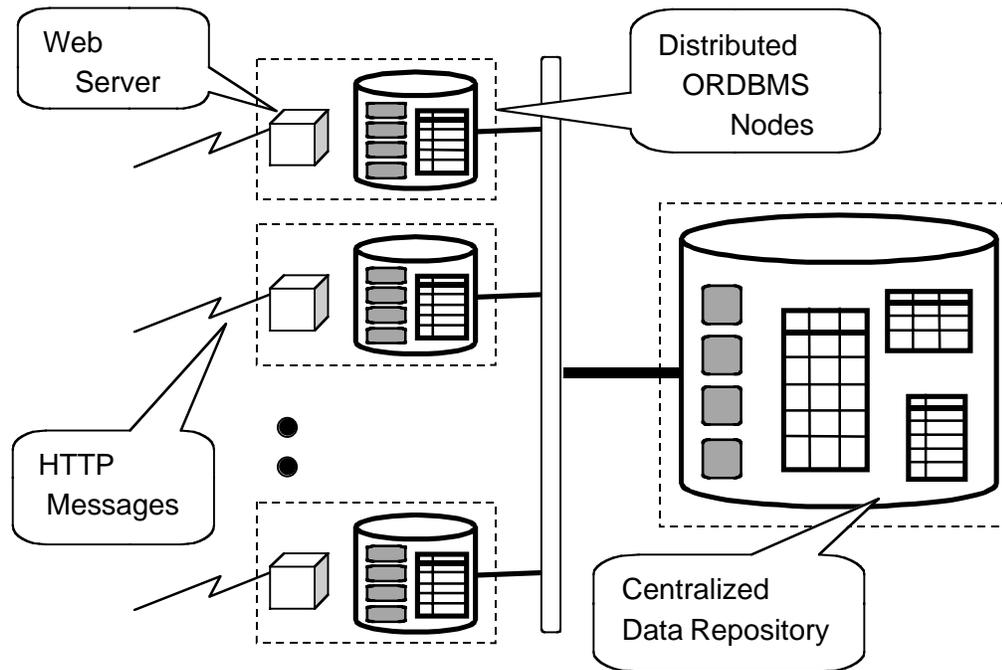
**Figure 1-7.** Distributed Information System Deployment
