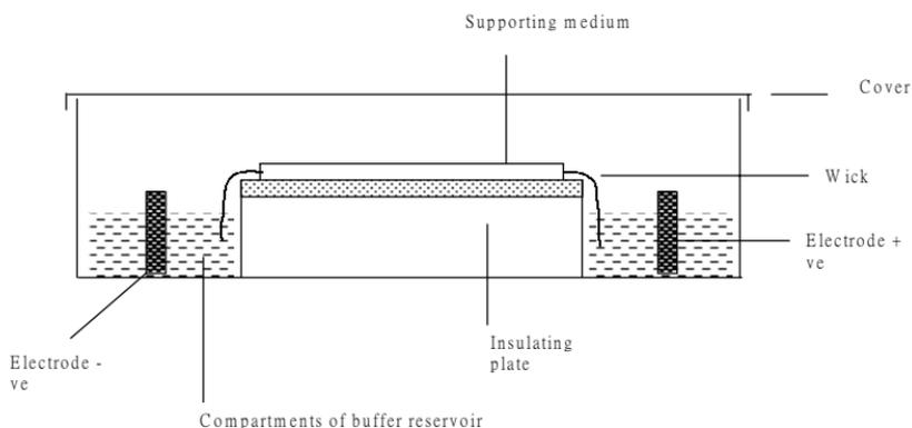
**Fig.10.6 An horizontal electrophoresis unit**
