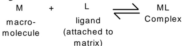
Under suitable experimental conditions when a complex mixture containing the specific compound to be purified is added to the insolubilised ligand generally contained in a chromatography column, only that compound will bind to the ligand. All the other compounds can be washed away and the compound subsequently recovered by displacement from the ligand. The purification of an enzyme by this technique is shown diagrammatically in Fig. 10.5.
