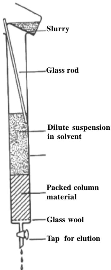
**Fig. 10.3** The preparation of a chromatography column
