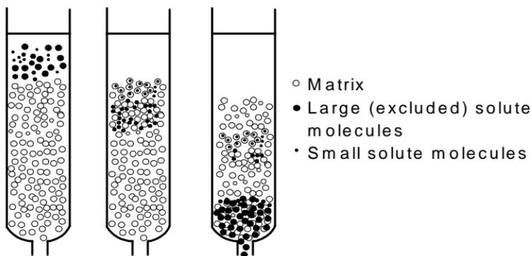
Fig. 10.4 Diagrammatic representation of separation by exclusive chromatography
