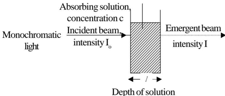
**Fig. 10.8** The absorption of light by a solution
