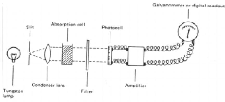
**Fig 10.9 A diagram of a photoelectric colorimeter**
