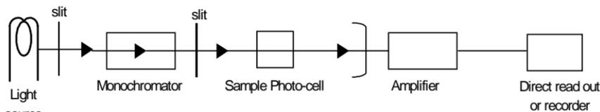
Fig. 10.10 The main components of a simple spectrophotometer
