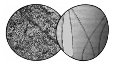
Fig. 6 - Microscopic Appearance of Viscose Rayon
