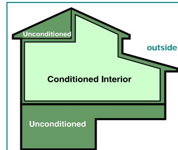
*The building envelope includes two elements: an air barrier and insulation that must be continuous and in contact with one another*
