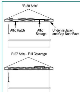
R-38 installed with 5% gaps or uninsulated areas yields the same heat loss as R-27 with full coverage - a 30% reduction!
