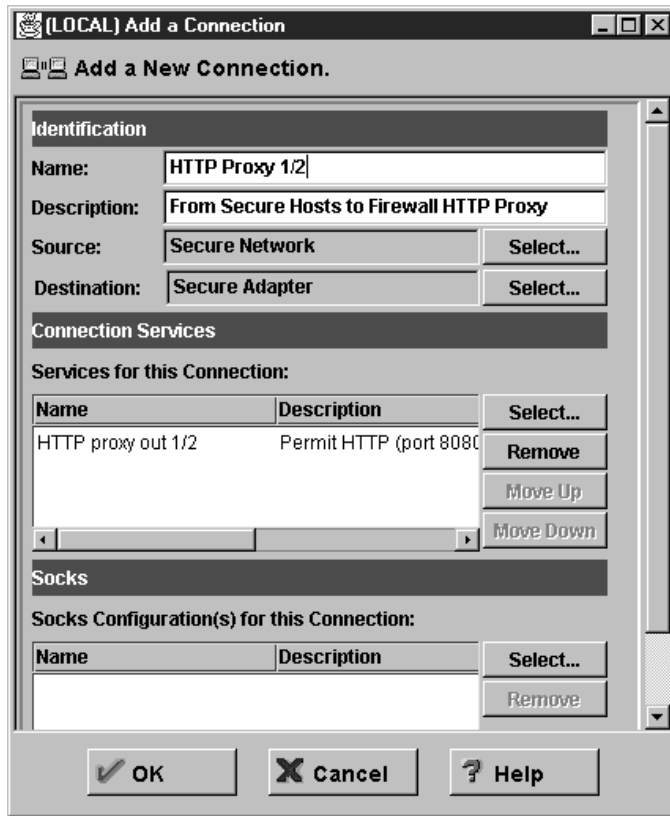
Figure 572. HTTP Proxy Connection on Secure Network
