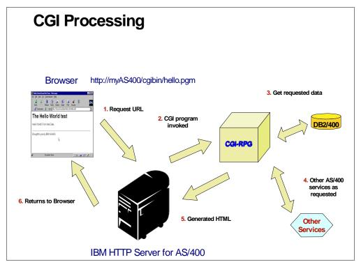
Figure 6. How CGI Processing Works
