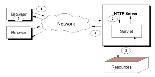
Figure 124. Servlet Architecture
