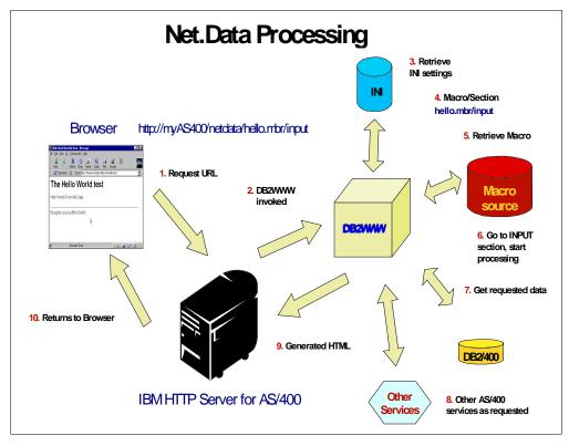
Figure 3. How Net.Data Processes a Macro and Generates a Response
