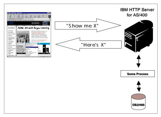
Figure 1. How an HTTP Server Processes a Request for a Dynamic Web Page
