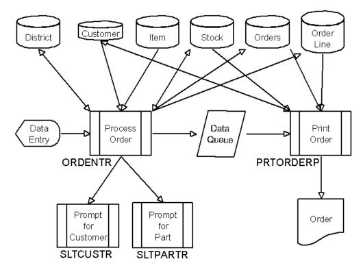
Figure 146. RPG Application Flow
