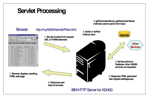
Figure 11. Servlet Processing
