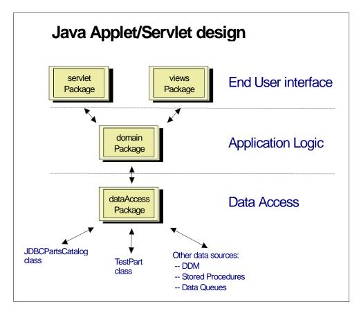
Figure 132. Java Applet/Servlet Design
