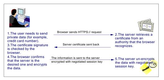
Figure 248. HTTP Server Using SSL
