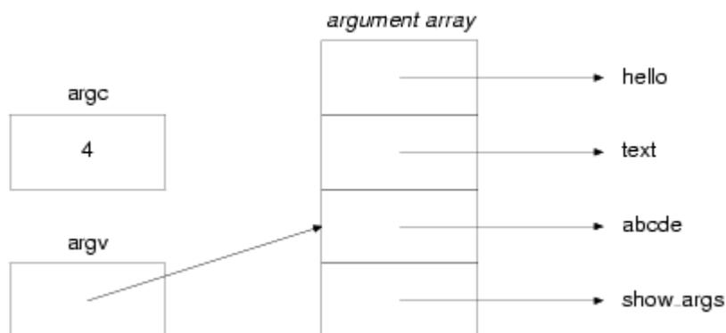
Figure 10.2. Arguments to a program after incrementing `argv`
